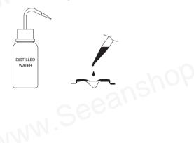
Press the ZERO key. If no error messages appear, your unit is calibrated. (For a description of error messages see "ERROR MESSAGES" section).
