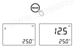
**Note:** The ATC tag blinks and automatic temperature compensation is disabled if the temperature exceeds the 10-40  $^{\circ}C$  / 50-104  $^{\circ}F$  range.
