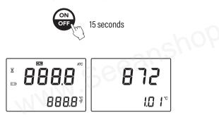
While continuing to hold the ON/OFF key, press the ZERO key. The temperature unit will change from °C to °F or vice versa.
