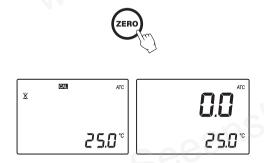
Gently absorb the ZERO water standard with a soft tissue. Use care not to scratch the prism surface. Wipe off the surface completely. The instrument is ready for sample measurement.
